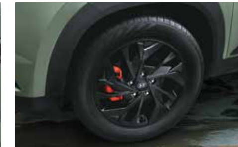
R17 (D=436.6 mm) black alloy with red front caliper
